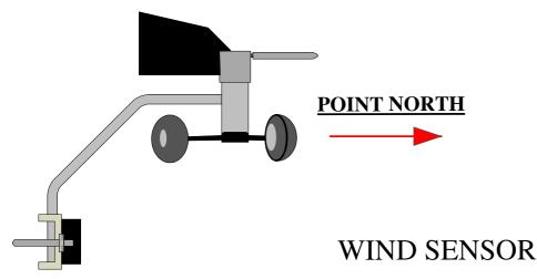
The combined Wind Speed and Direction Sensors are manufactured from anodized aluminium alloy, uPVC and stainless steel with moulded polypropylene cups. The units are lightweight (less than 250 grammes) yet very robust.
