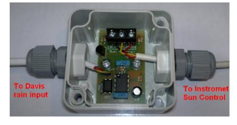
Once this has been done, the 50cm RJ11 plug can then be connected to the Davis "rain sensor" input. Ensure the Davis Rain input is set to 0.01" to get the correct sunshine reading when the system is running.
