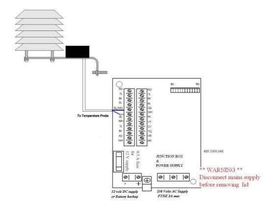
Wall or mast mount away from heater or air conditioner outlets. Avoid mounting over flat roofs which may radiate heat during sunny periods.
