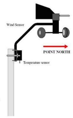
Mast mount 25-50mm dia. or Instromet mast kit Long 480 1000 096 Short 480 1000 103 Tile/slate clamp 480 1000 097
